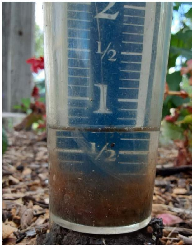
Reading from a local rain gauge. Approximately 3/4" of rain during this monitoring event. This reading stands on its own and a SWPPP inspection must be completed by the end of the next business day.
